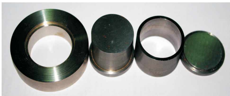
Rys. 3. Metalowa matryca do pastylek \varnothing = 37 mm
