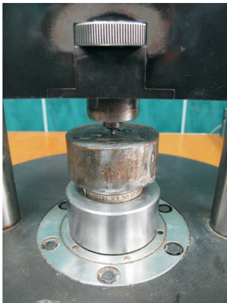
Fig. 1. Cylindrical indenter acting on the sample [6]
