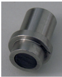
Fig. 2. Nozzle with the grease for the flow pressure of lubricating greases test (photo: INiG – PIB)
