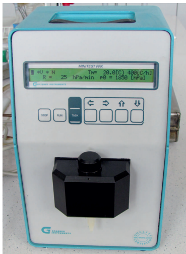
Fig. 3. Apparatus for the flow pressure of lubricating greases test (photo: INiG – PIB)
