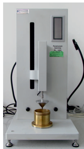
Fig. 1. Penetrometer for determination of grease penetration (photo: INiG – PIB)
