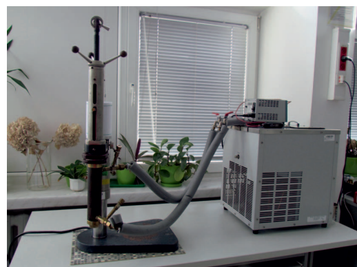
Fig. 4. Capillary tube for determination of apparent viscosity of the greases (photo: INiG – PIB)
