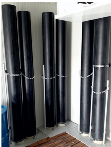
Fig. 1. Test stands for diesel fuel storage (photo: INiG – PIB)
