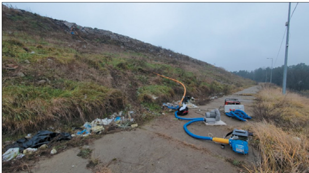
Figure 1. The set for dynamical reception of landfill gas from a landfill
